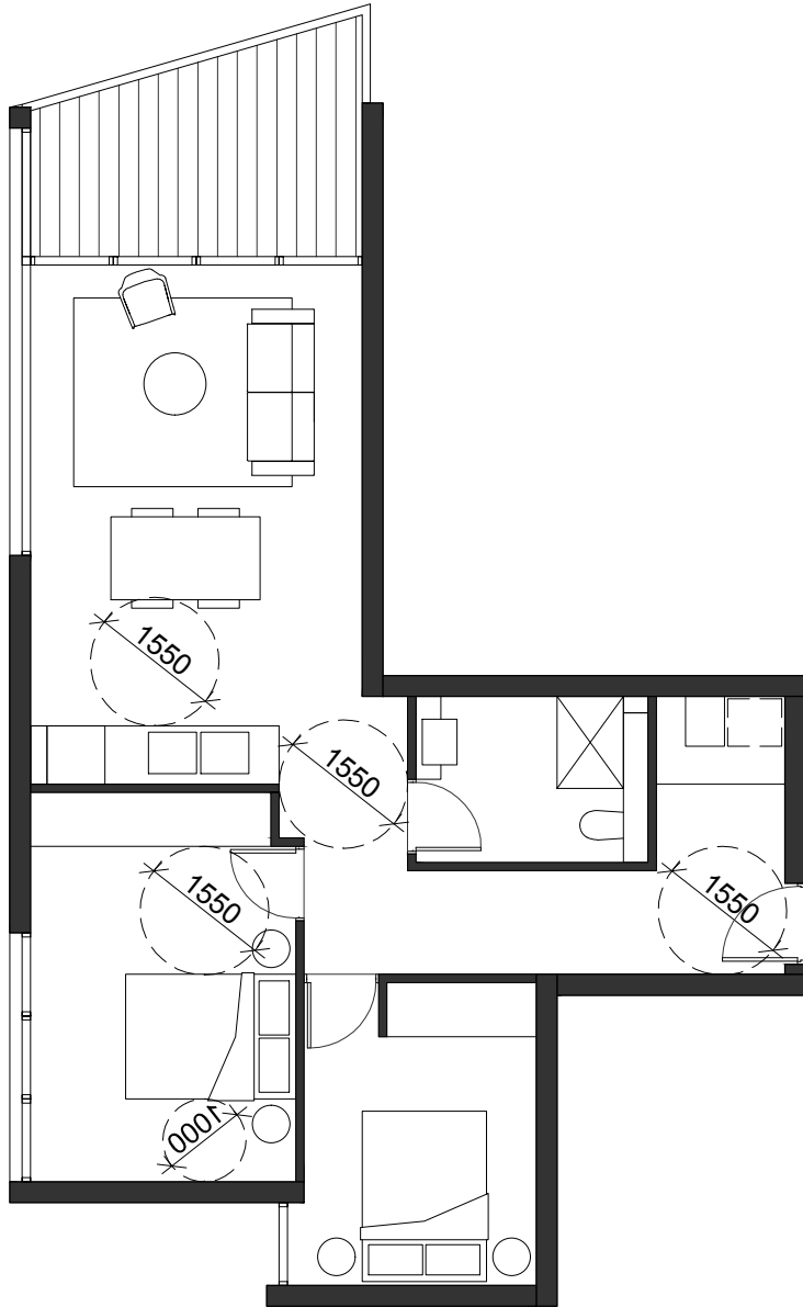
ADAPTABLE TWO BED ROOM UNIT - 70m 2 B.2.01,B.3.01,B.4.01
